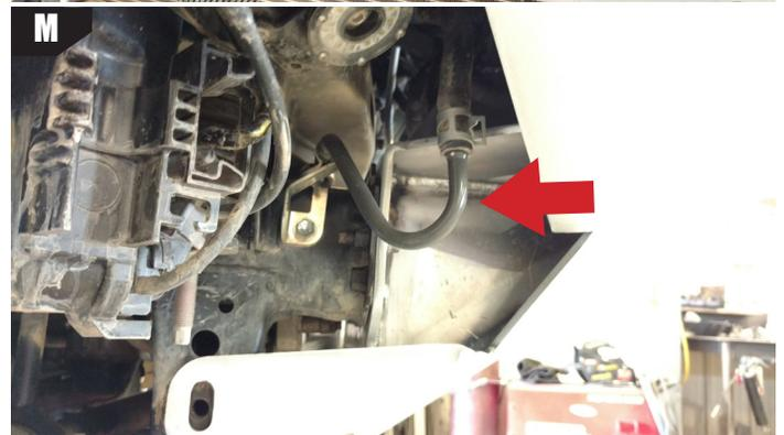
8) Cut the plastic mounting that the bumper clips into on the sides even with the original cut. Do not cut too deep, the metal pinch weld will stay.
