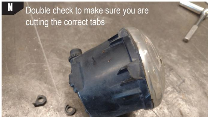
**N** Double check to make sure you are cutting the correct tabs
