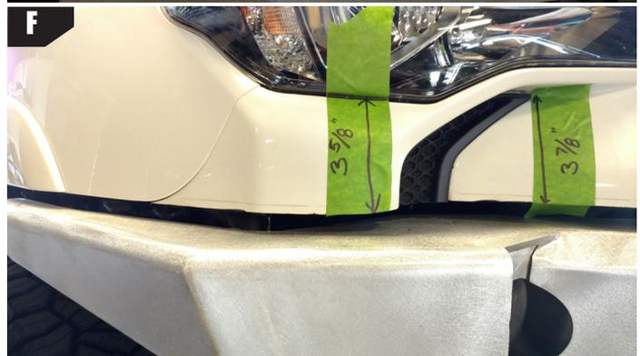
stretch a piece of masking tape around the bumper on each side to middle grill, (a laser can be helpful with this step, they can be found inexpensive at Harbor Freight). **Photo – G** shows where to cut the grill. Once the cut is complete the bottom half of the bumper should fall off.
