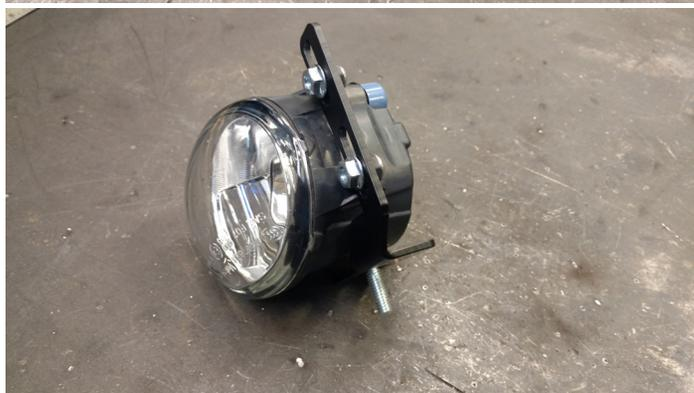
You can now bolt this assembly into the bumper and adjust. The CBI Premium bumper accepts most modern winches. If mounting a winch, now is the time before the bumper is mounted to the truck. **NOTE: if mounting a winch leave the center plate off the bumper with the fairlead, this will be installed later.**
