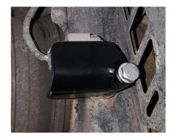
**2.** For the rear guards, remove the 10mm nut holding the sensor. Pull the sensor out and remove the factory stud. Install the guard on the appropriate side using the provided hardware and adjust so the bottom plate is parallel to the ground and tighten.
