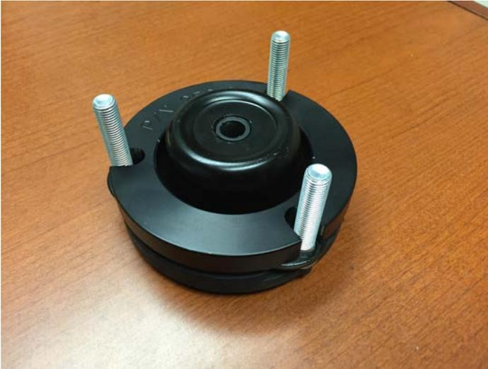
19. Position the coilover onto the vehicle, sliding the top into the shock tower first. Install the top three nuts which hold the coilover to the shock tower finger tight. Install the lower shock bolt and nut. **You may need to pry down on the upper control arm in order to get the lower shock bolt installed.** Torque upper nuts and lower bolt/nut to manufacture specs.
