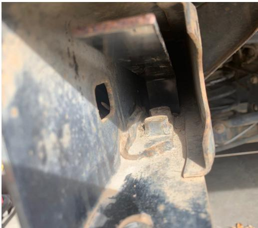
4. Place assembled bumper onto frame rails and align with holes in frame. Install the nut plate bolts first so they don't get knocked out of alignment with the frame holes. Tighten up remaining bolts.
