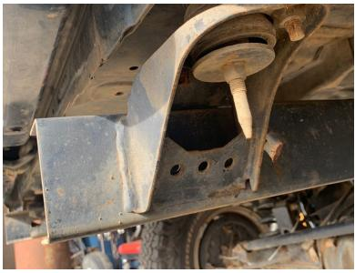
3. Install nut plates in the frame so they line up with the two furthest mounting bolt holes inside the frame.
